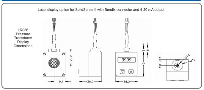
The SolidSense II pressure transducer is available with an optional display: Model LR056, for details on this display see **DS-PR-LR056-eng**
