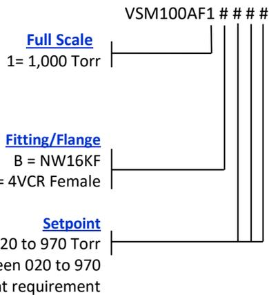
Example: VSM100AF1G030 (Absolute vacuum switch with 4VCR fitting, setpoint at 30 Torr)
