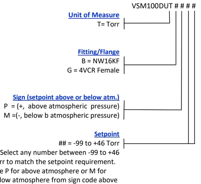
Example: VSM100DUTGP40 (Differential vacuum switch, Torr, 4VCR fitting, setpoint 40 Torr above atmospheric pressure)
