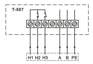
H1, H2 and H3 are alarm signal output terminal; A,B and PE are MODBUS RS-485 communication output terminal.
