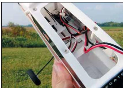
*Megatech's new four-channel transmitter is provided, and all the airborne gear is factory installed.*
